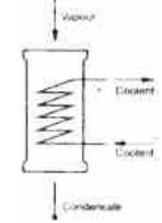
This method produce a cool condensate using the entire cooling surface area. This method should be used where the condensate can lead to "logging" of coils.
