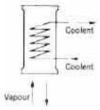
This method is simple to install over a reactor. However this results in condensate returning substantially at its condensing temperature. In this method care must be taken that condensate is not excessive that it can lead to "logging" the coils and create back pressure in the system. Generally a reflux divider is used below the condenser to take out the distillate.
