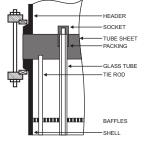
The shell side is made of baffle which provide large heat transfer area, while the tubes are inserted in the shell through PTFE Plates & proper packing, which makes it easier for cleaning & removing.
